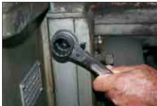
Ratchet podgers: For extra leverage on fasteners in confined spaces.
