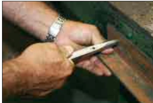
Ratchet podgers: Align bolt holes easily.
