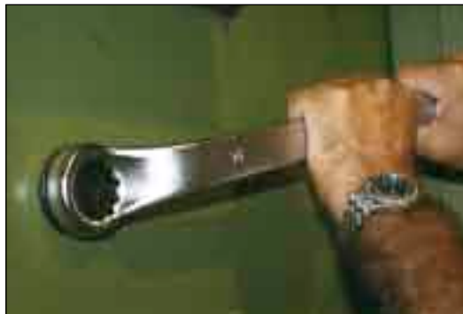
Ring podgers: Where extra leverage on tough fasteners is required. Ring podgers: Align bolt holes easily.
