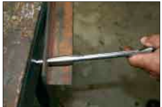
Ring podgers: Where extra leverage on tough fasteners is required. Ring podgers: Align bolt holes easily.
